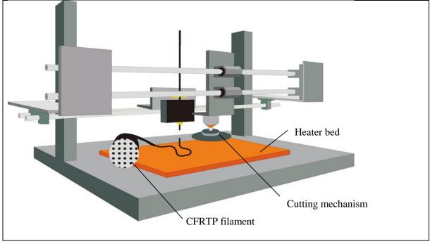
Figure 1: Schematic diagram of the 3Dprinter with continuous carbon fiber and cutting mechanism.
